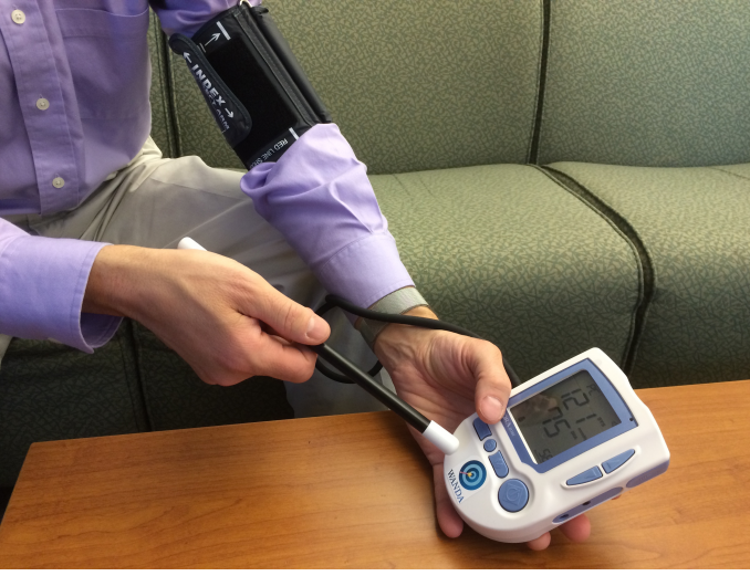
Fig. 4. Blood pressure monitor with Wanda logo indicating where to place the Wand.
