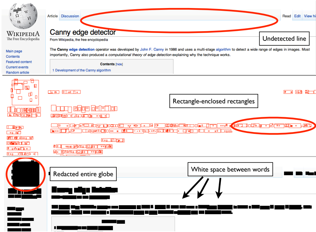
Figure 2: Canny-based text redaction. The top image is a screenshot snippet from the Wikipedia page about Canny edge detection [17] (recall that contractual obligations prevent us from disclosing the EMR screenshots we tested on). The second image depicts the rectangles that result from processing the first image with Canny edge detection, polygon detection, and polygon bounding with rectangles. The third image derives from filling the rectangles in the second image and then applying the second image as a redaction mask to the first. Canny missed some true edges throughout the image (false negatives for edge detection) and added edges where text does not exist near the globe (false positive for text detection). Finally, notice whitespace between words and tiny rectangles enclosed within larger ones.
