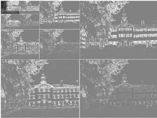
Figure 3: Shown are the absolute values of the subband coefficients at three scales and three orientations for an image of Dartmouth Hall, Figure 2. The residual lowpass subband is shown in the upper-left corner.
