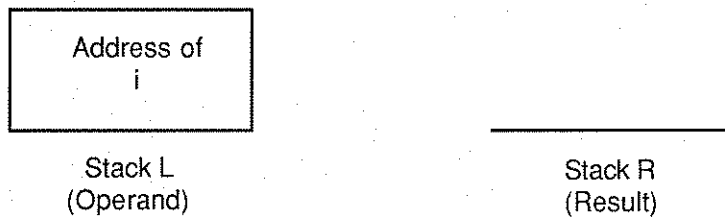
Figure 10: Stack Switching -- After First Operand is Stacked
