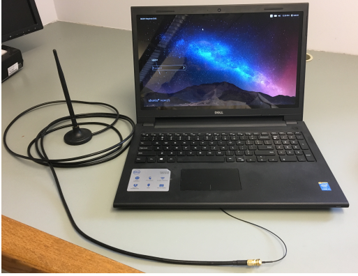
Figure 8: Transmitters. We used a quarter-wavelength and a half-wavelength dipole antenna as well as a micropatch antenna connected via a 3 m cable to an internal Intel Ultimate N WiFi Link 5300 adapter installed in a Linux laptop. We also used a Panda Ultra Wireless N USB adapter connected via a 1 m USB cable.
