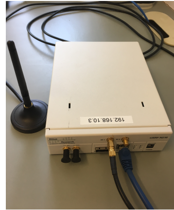
Figure 7: Receiver. We used a USRP 210N Software Defined Radio with a quarter-wavelength dipole antenna as a Wi-Fi receiver. The USRP was connected to the antenna via a 3 m RF cable and to a laptop via a 2 m ethernet cable (laptop not shown).
