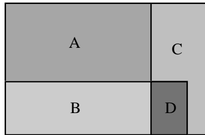
fig 17. Example of the region growing overlap problem. A is a region that has finished growing. B and C are two child regions. If both B and C are not restricted, the overlap region D is possible.
