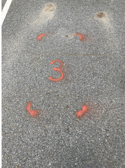
Figure 4.12: Close up of spot #3. We marked four corners to designate the placement of the sensor board. This ensured the sensor board was placed in the same location for each reading.
