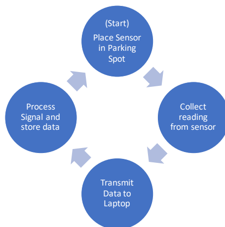
Figure 4.1: Radio communications. Sensors placed in parking spot measure magnetic data and transmit the data over an NRF24L01 radio to a laptop for analysis.
