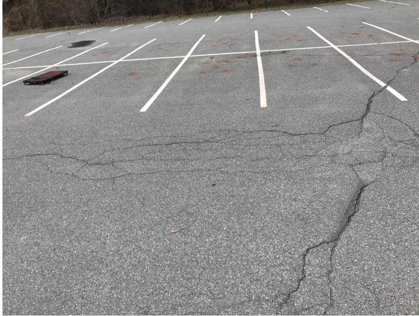
Figure 4.10: Collection of baseline readings. The sensor board can be seen on the left side of the picture as well as the spray painted marks denoting the space number and the sensor board placement.
