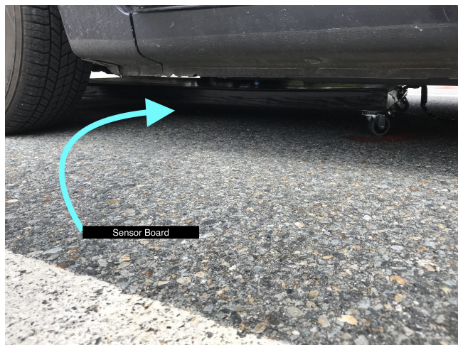
Figure 4.13: We placed the sensor board under vehicles, lining up the board with the spray painted markings.
