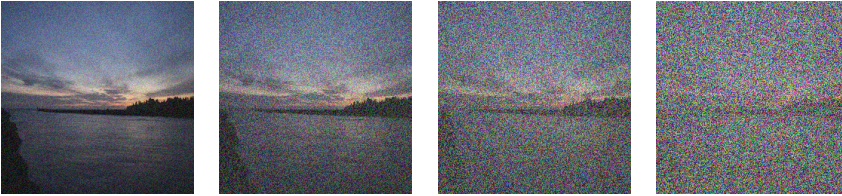
Figure 4: Degraded images with noised added. P values of 0.2, 0.4, 0.6, and 0.8 were used to determine how much noise to add to the image. Images are shown in order from least noise added to most noise added.
