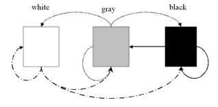
With this, any live object graph structure must be marked, and upon completion of collection, this structure must reside completely in the black region to avoid loss of live objects.
