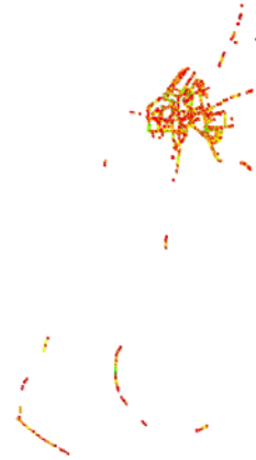
Figure 5: Netstumbler output is projected in the UTM Zone 18N coordinate system. ARCGis reads in the text or dbf file, and spatially projects the data with the desired symbology. The dots represent points where netstumbler recorded wireless activity; Here a red dot means poor signal strength, and green is strong signal. The dots provide a breadcrumb trail showing where the scanner was driving/walking.
