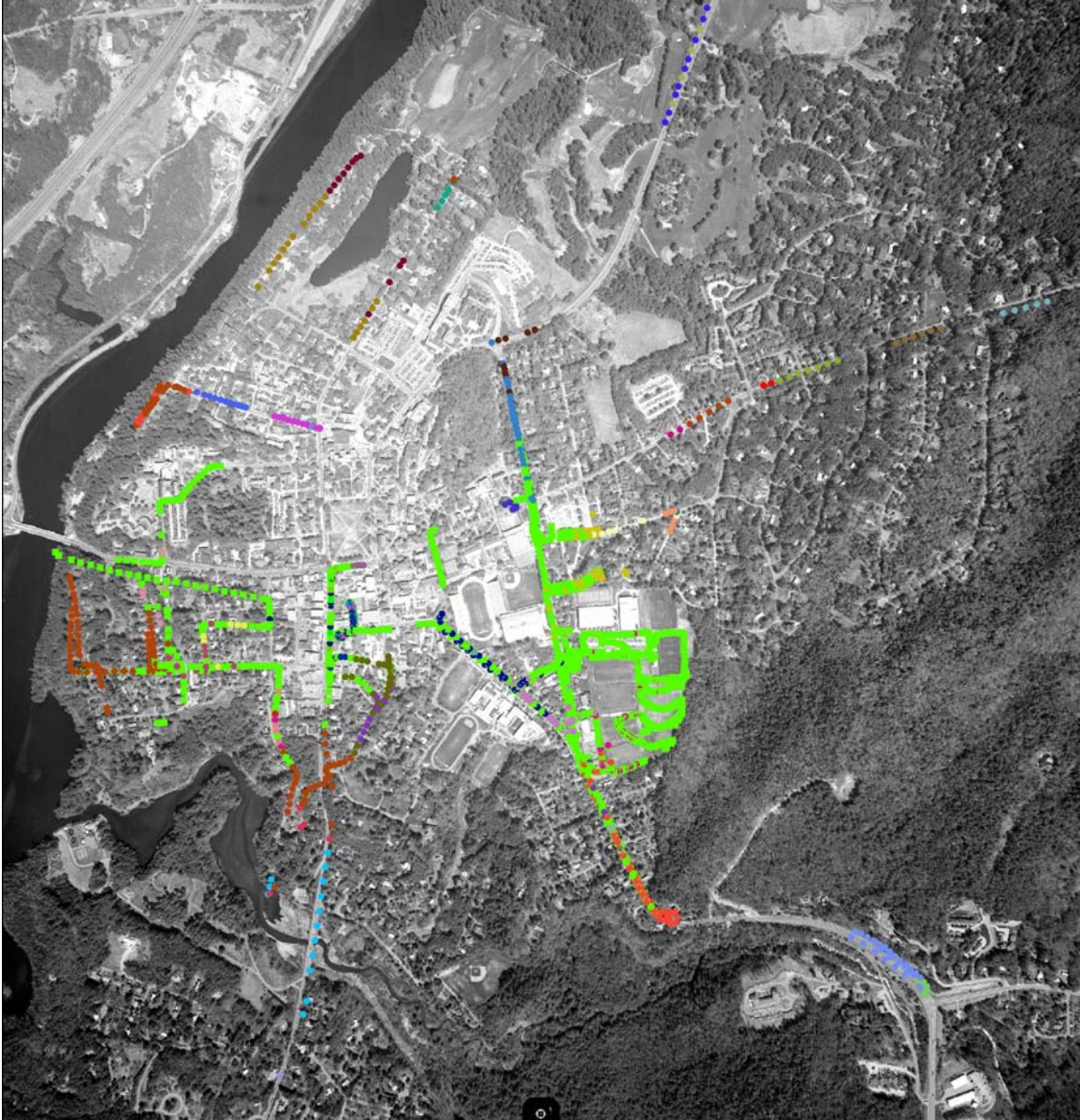
Map 1: Driving Tour of the wireless networks in Hanover NH. This is a map of every network in Hanover that broadcasts its SSID. Each dot represents a Signal to Noise Ratio reading > 5 dB. Different SSIDs are drawn in different colors; The green squares are readings from the Greenwave Wireless network, the off-campus network I am deploying.
