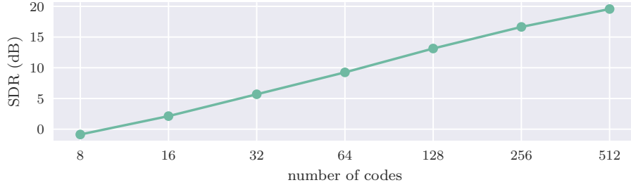
Figure 5.3: Complex Conditional VQ. SDR for different values of N (number of codes) and a fixed code size of K = 4 .
