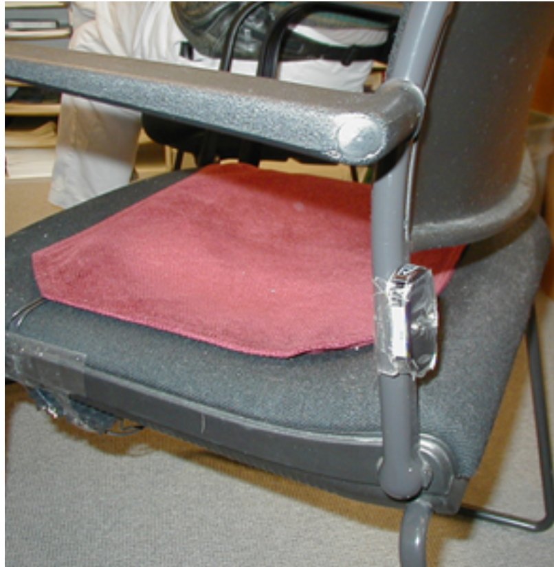
Figure 2.3: An instrumented chair with a wireless pressure (placed in the seat mat) and a motion sensor (taped at the back of the chair).
