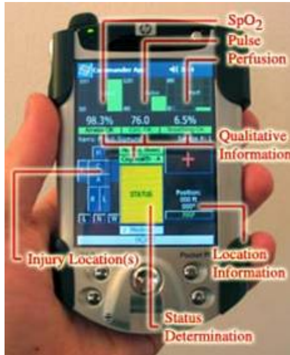
Figure 7.10: A front-end application running on the mobile device carried by first responders.
