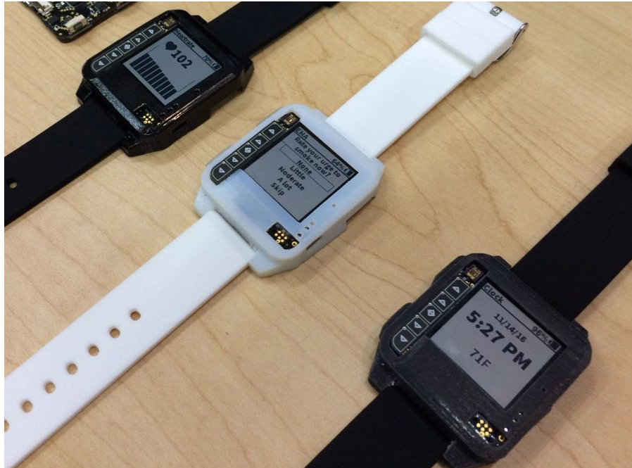
Figure 2: Amulet prototypes running various apps: heart rate app(left), EMA app (middle) and clock app (right)
