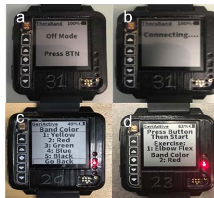
Fig. 4 (a) Snapshot of TheraBand application states: Off (a); Connection (b); View of band color (c); Initiation of Exercise (d)
