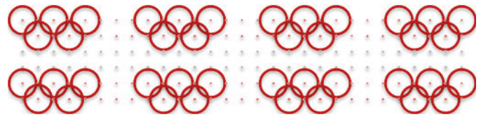
Fig. 8. Alignment of the rings to get a structure, where the rings are arranged like on the Olympic logo. Each position (representing a pulse) is equidistant with a distance of 150 \mu\text{m} in X- and Y-axis. Selectively blanking out single pulses forth and back direction results in the desired structure.
