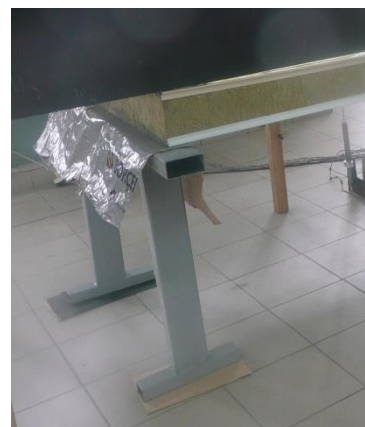
Fig. 5. Supports – special metal structures (jacks).
