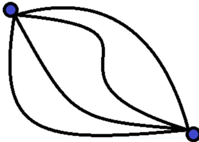
Fig 1. A schematic representation of an origin-destination network. Blue dots represent the origin and the destination nodes. Connections between them represent the ensemble of pathways described by the probability distribution \{p_c\}_{c=1}^C . The CR family allows one to determine the probability coefficients p_c , \forall c by making use of the available partial information, i.e. aggregate data on traffic volumes.
