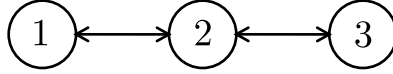
Figure 2.1: The graph depicts the communication structure of the three-player chain problem. Edge weights (not shown) indicate the delay required to transmit information between nodes.
