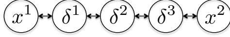
Figure 3.1: The distributed plant considered in (3.6), shown here for D = 4 . Dummy nodes \delta_t^i , i = 1, \dots, D - 1 , as defined by (3.5), are introduced to make explicit the propagation delay of D between plants.
