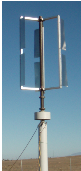
Figure 5.8. Flexible blade turbine with stainless steel blades.
