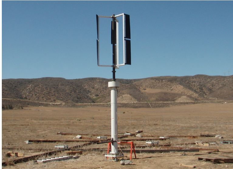
Figure 5.5. Flexible blade turbine with rubber blades.
