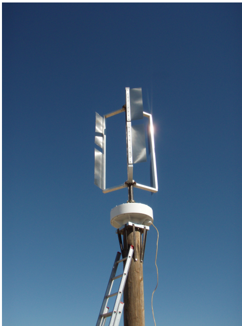
Figure 5.10. Stainless Steel Blade Turbine on high torque generator.
