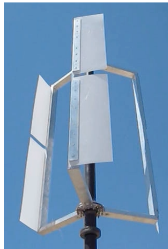
(b) Turbine with 1/32 inch thick Delrin blades installed. Image courtesy of davidkremer
