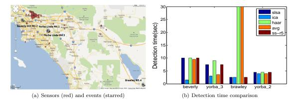
Figure 5.18: CSN network. (a) plots the layout of 128 sensors and epicenter of 4 recorded events. (b) The learned bases detect on average several seconds faster than the baselines under the constraint of at most one false alarm a year.
