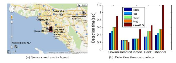
Figure 5.19: Long Beach array. (a) shows the layout of 1,000 stations and 5 recorded events. (b) Under the constraint of at most one false alarm a year, the learned bases detect on average 0.1 seconds faster than the baselines, which is significant considering it only takes 1 second for the seismic wave to travel through the network and only 0.5 seconds for the network to be saturated with signals.
