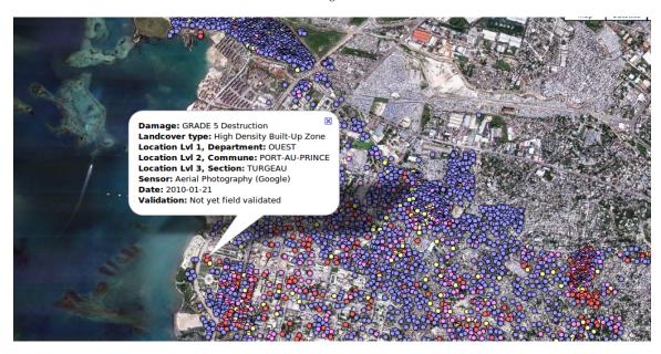
Figure 1.2: A satellite-based damage map from Haiti, following the January 12, 2010 earthquake, depicts localized variation in damage. Sensors could provide such information to emergency teams without waiting for aerial photos. Image provided by Google.
