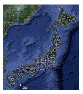
Figure 5.15: There are approximately 1,000 ( $\approx 1$  per 20  $km^2$ ) seismic stations that observe and record on average 500+ seismic events that occur in Japan each day. Among those 1,000 stations,  $\approx 800$  are *Hi-net* stations, pictured here. These research-grade sensors are professionally installed and maintained and therefore experience very little instrument or ambient noise.
