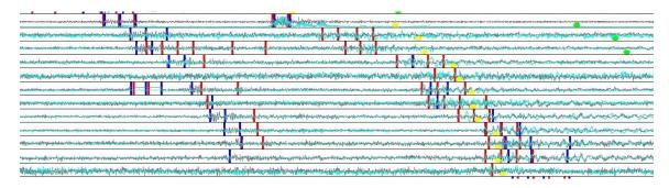
Figure 4.2: CSN sensors produced picks (blue and red bars) for both P-wave and S-wave of the Anza M3.6 earthquake. Time series plots are arranged by distance to quake epicenter.
