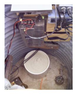
Figure 2.1: A CISN sensor station installed in a "borehole". Installing and maintaining such stations represents significant investment, but provides exceptional quality.
