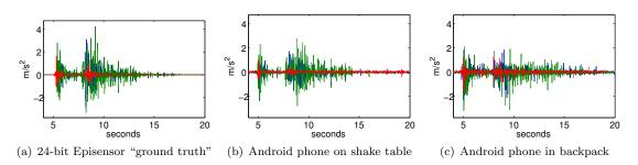
Figure 3.5: Android accelerometers accurately record strong shaking during a shake table experiment. (a) Ground truth. (b) Android phone. (c) Android phone in backpack.
