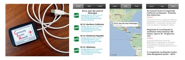
Figure 1.1: CSN volunteers contribute data from low-cost accelerometers (left) and from Android smartphones via the CSN app *CrowdShake* (right).
