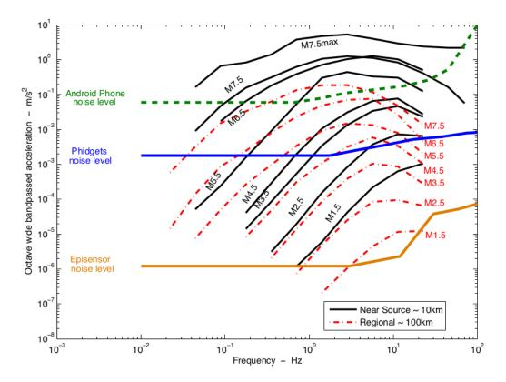
Figure 3.6: The accelerometers in smartphones (e.g., Android) and USB sensors (e.g., 16-bit Phidget accelerometers) are capable of sensing moderately large earthquakes. Scientific-quality sensors (e.g., the 24-bit Episensor) are capable of measuring quakes well below the level of human perception. Figure courtesy of Ming Hei Cheng.
