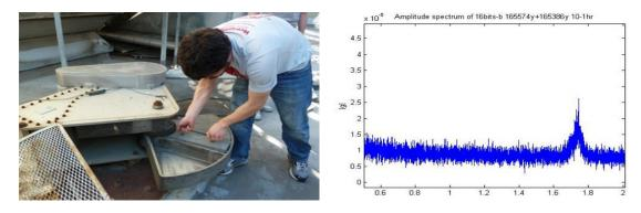
Figure 3.7: Eccentric weights oscillate Millikan Library, demonstrating that CSN hardware can observe resonant frequencies in buildings.
