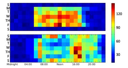
Figure 5.9: Even simple statistics such as pick rates can reveal patterns of activity and occupancy in the area around a sensor. A Phidget sensor in an office setting (above) shows high ambient noise (human activity) during weekday business hours, while a Phidget in a home (below) shows typical evening and weekend activity.
