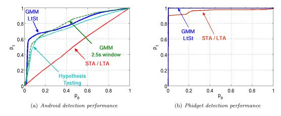
Figure 4.3: In all plots, the system-level false positive rate is constrained to 1 per year and the achievable detection performance is shown. (a,b) Sensor level ROC curves on magnitude M5-5.5 events, for Android (a) and Phidget (b) sensors.
