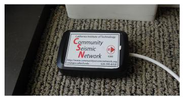
(b) "Phidget USB accelerometer"
