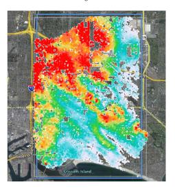
Figure 1.3: A map of peak acceleration amplitudes experienced in Long Beach, California during the Carson earthquake, as recorded by Signal Hill Petroleum. The map shows large variations in peak acceleration and the effects of a minor fault line.
