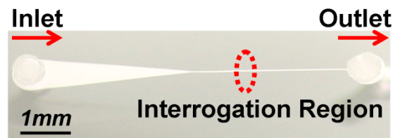
Figure 2.9. Photos of (a) the fabricated microfluidic device and (b) a zoomed-in photo of the fluidic channel.
