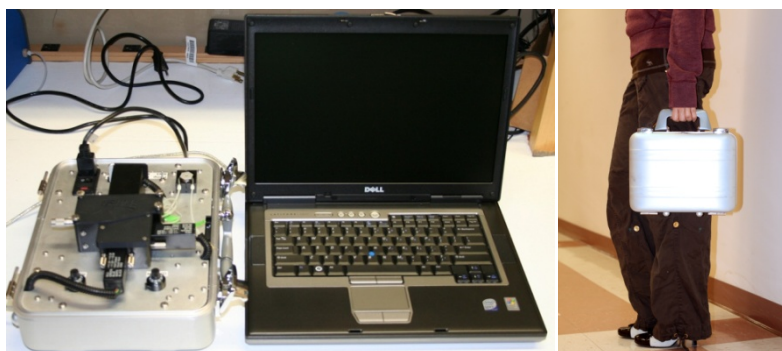
Figure 5.2. The test platform configuration of the microfluidic cytometer. (a) The optical system was used together with a laptop computer, and (b) the system was packaged into a suitcase for being carried around.
