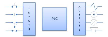
Figure 2.9: PLC main parts
