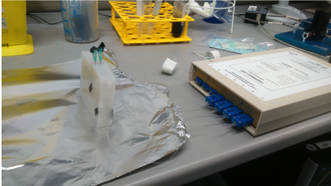
FIGURE 3.10: Thermocouples connected to DAQ 'Thermes Usb' (Physitemp)
