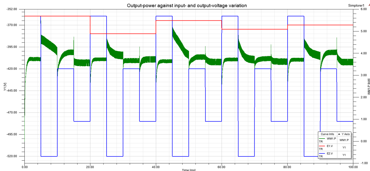
Figure 3.32 Output-power response against input/output-voltage variation
