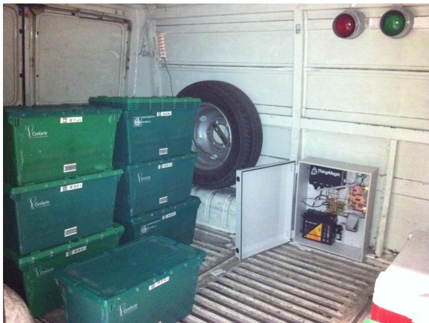
Figure 13. Onboard system deployed on a vehicle. The transport bins of green color with the corresponding RFID tags can be seen on the left hand side of the picture.
