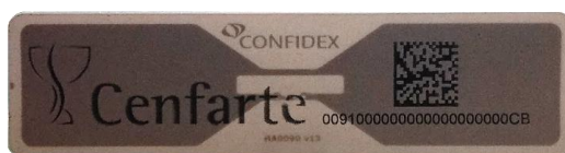
Figure 2. Confidex's Carrier Tough passive tag.
