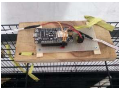
Figure 5. The design of the NODE MCU on PCB Board
