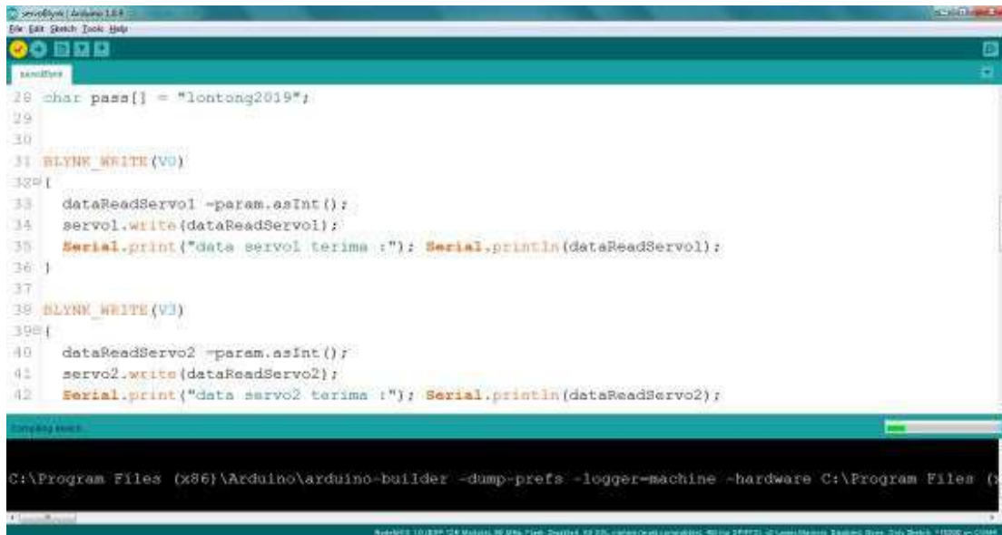
Figure 8. The process of Uploading Data from the Arduino IDE to the ESP8266 Chip
