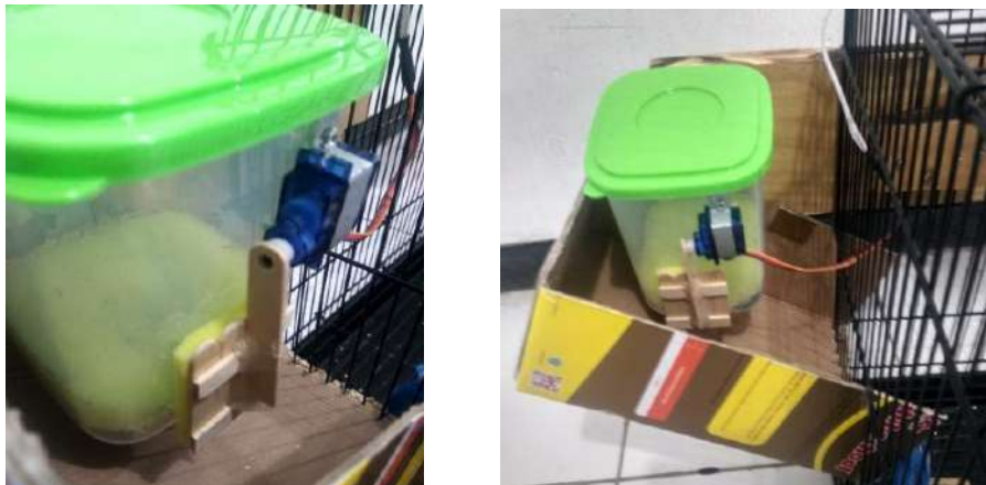
Figure 6. Installation of bird feeding valve
