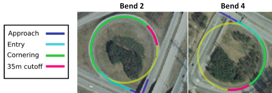
Fig 4. Segmentation of the analyzed bends. Approach, Entry, and Cornering phases were identified based on visually identifying the change in bend curvature from the aerial image. Note that the cornering phase of bend 2 is about twice the length of bend 4. The yellow arcs that complete the circles are included to indicate that the cornering section adheres to constant curvature. The curve radii are approximately 48m.
