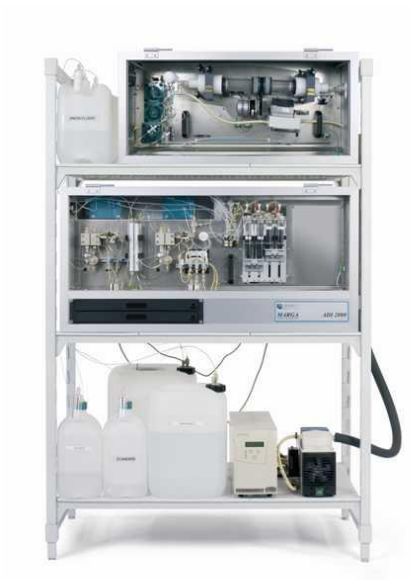
Figure 4. MARGA 1S (Monitor for AeRosols and Gases in Air).
