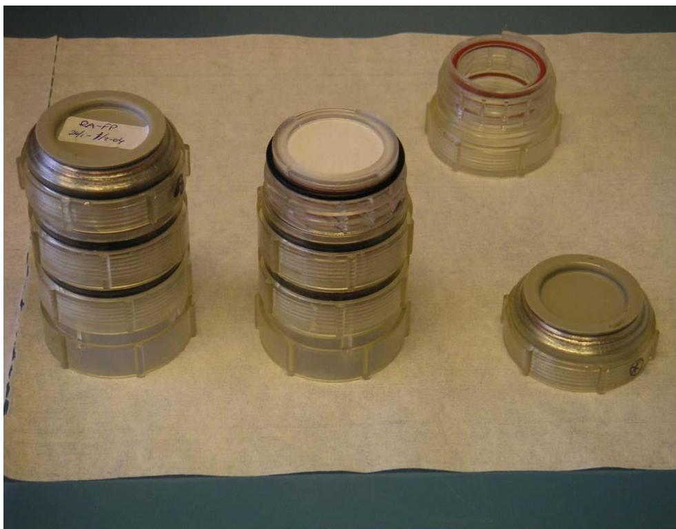
Figure 2. EMEP 3-stage filter packs (NILU Products, Norway).
