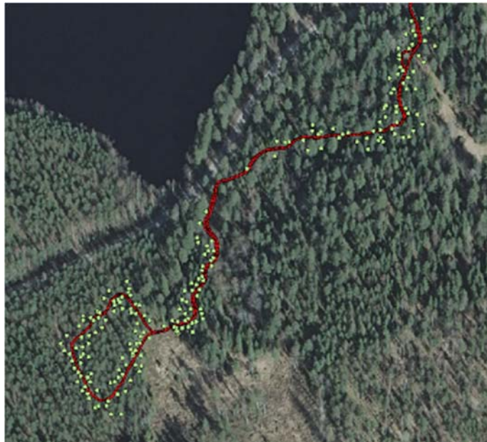
Figure 2. The reference trajectory (red) and the reference trees (green). Background orthoimage: National Land Survey Finland 2012.
