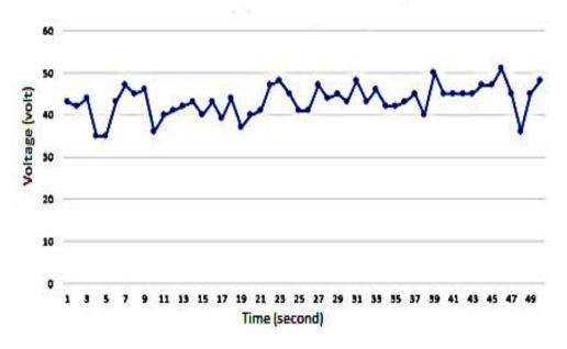
Figure 5. Voltages generated by 40 piezoelectrics in parallel
