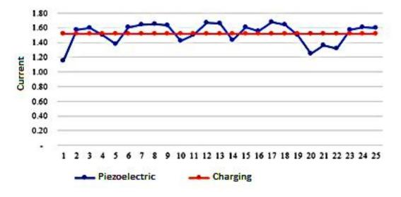
Figure 8. AA battery test using 40 piezoelectrics in parallel
