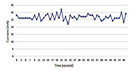
Figure 6. Current generated by 40 piezoelectrics in parallel
