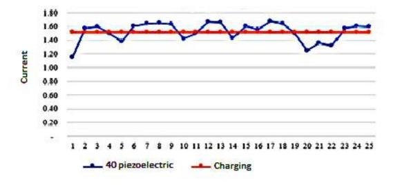
Figure 7. AA battery test using 40 piezoelectrics in parallel
