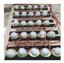
Figure 2. The 40 piezoelectric circuit is coupled by using a parallel circuit
