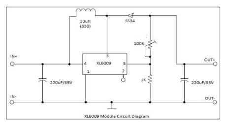
Figure 3. Boost up converter circuit
