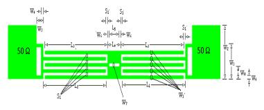
Figure 1. Configuration of the proposed UWB BPF with rectangular slot at input/output port
