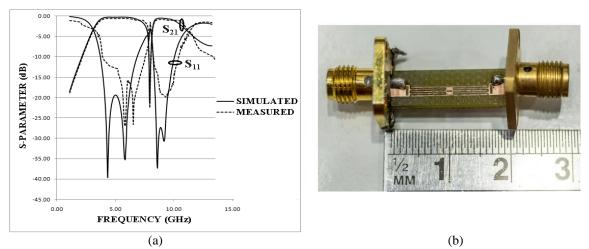
Figure 5 (a) Comparison between simulated & measured. (b) Photograph of the fabricated filter
