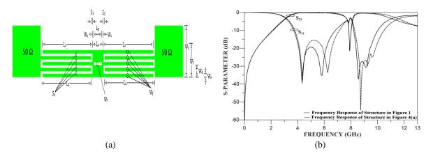
Figure 4 (a) Proposed filter without rectangular slot at input/output port. (b) S-parameter of Proposed filter with and without rectangular slot
