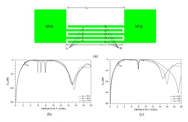
Figure 3 (a) Layout of the coupling structure. (b) L2 is kept constant and L1 is varied. (c) L1 is kept constant and L2 is varied
