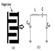
Figure 2. Interdigital Structure (a) Layout (b) Equivalent circuit
