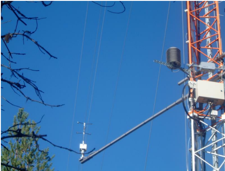
Figure 21. The Gill sonic anemometers have been replaced by ice-free Metek 3D sensors. The one in the figure is placed at 2 m height close to the mast to measure fluxes close to the ground.
