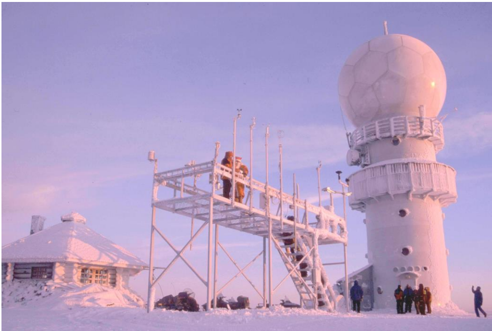
Figure 7. The FMI Luosto weather radar with the testing site for studying the impact of icing upon meteorological sensors visited by Santa Claus (standing on the test platform).
