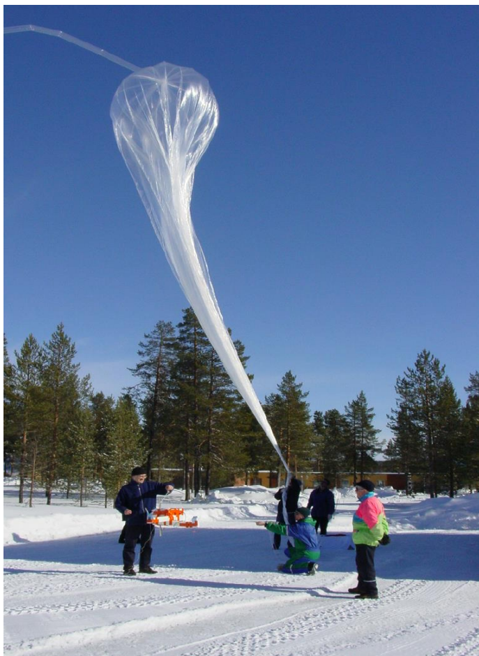
Figure 30. Balloon launch at FMI-ARC. In addition to conventional sensors this payload is also equipped with ozone measurement sensors.
