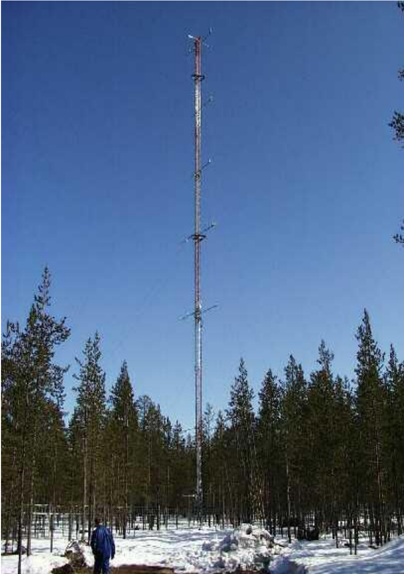
Figure 18. The 48m-meteorological mast (shown here in winter time) is an example of an inter-discipline research tool. The mast is used e.g., for measuring the exchange of carbon dioxide between vegetation and the atmosphere.
