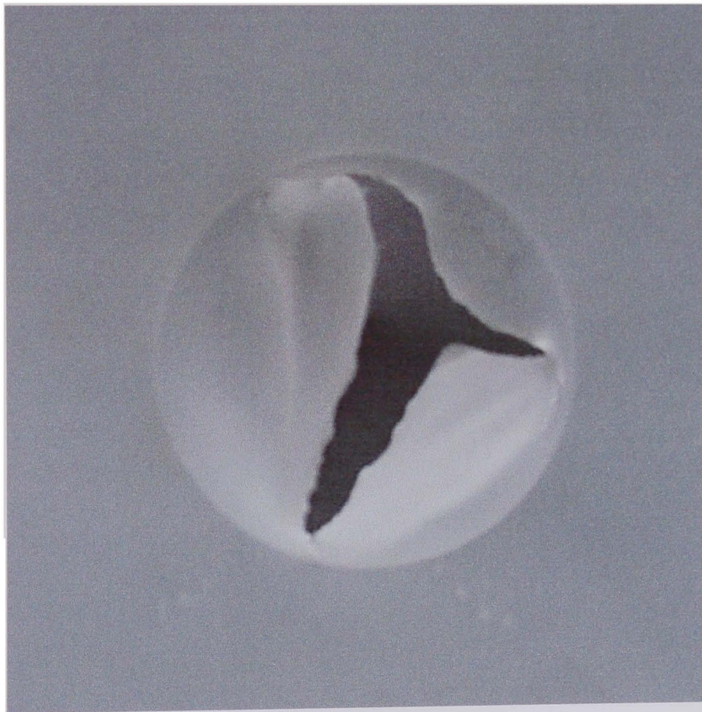
Figure 5.8 – Punctured diaphragm material.
