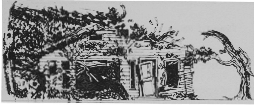
Figure 2.2 – B. Immediately after the passage of the shock front. The force experienced by the object is proportional to the pressure rise and the impact area.
