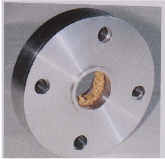
Figure 5.13 – Ceramic foam holder for Sample 1.
