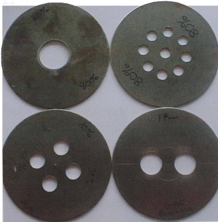
Figure 5.22 – Orifice plate configurations (80% BA).
