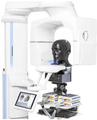
Fig. 3.5.1 The MOSFET measurement setup with four TN-RD-16 reader modules, RANDO phantom, and a ProMax 3D MID CBCT device (I).
