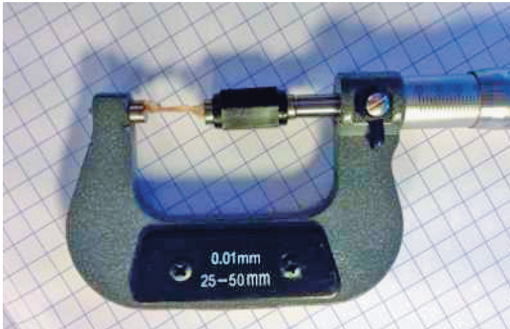
Figure 13. Measurement of femur length. Femur length was measured from the fixed right femur of each mouse using a micrometer.
