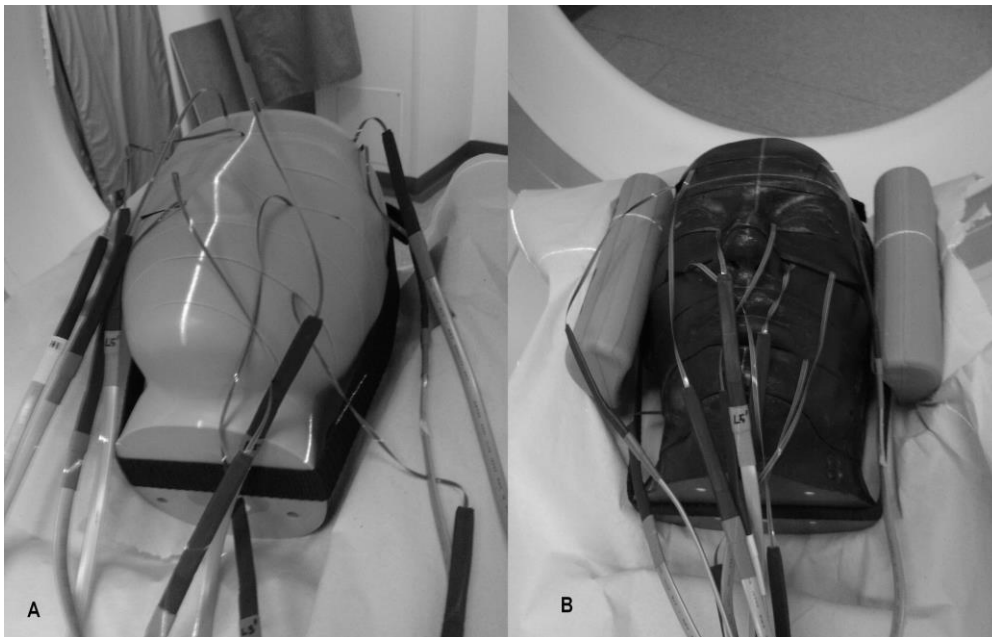
Figure 3 Anthropomorphic head phantoms used to assess radiation exposure to the eye lenses in a routine head CT. a) ATOM Model 703-D, b) RANDO (Study IV).
