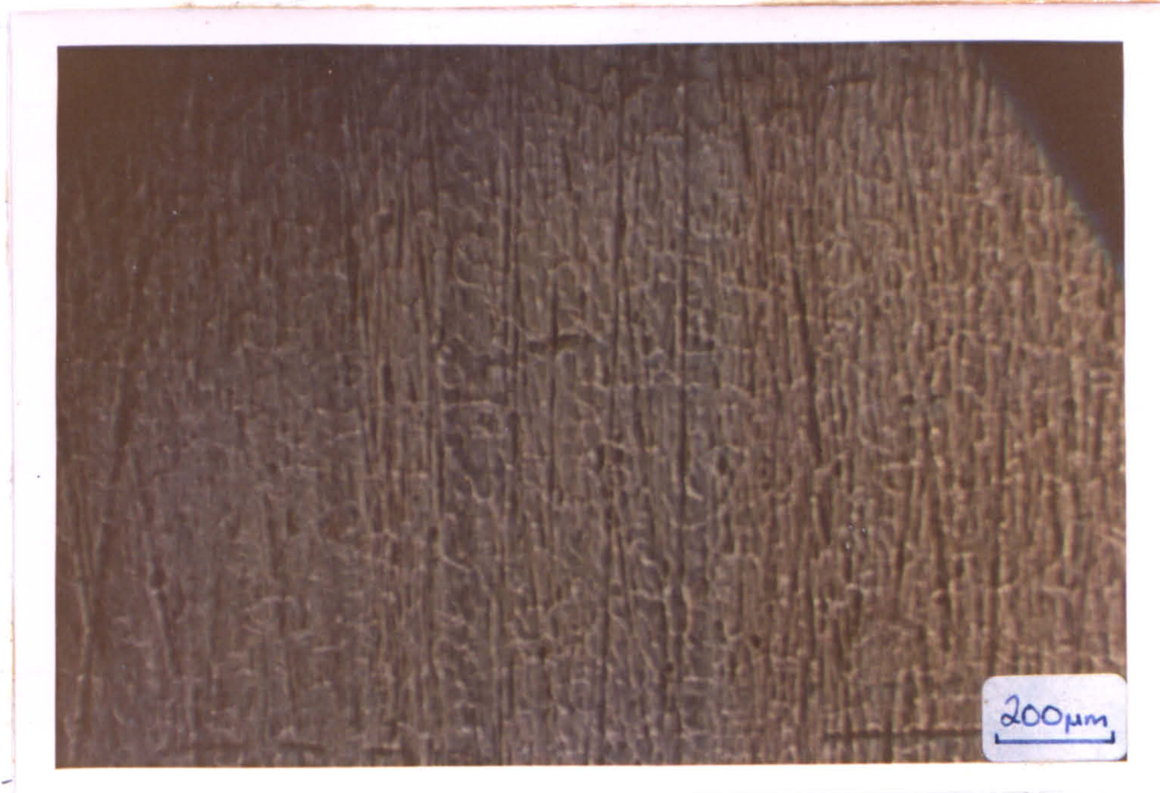
FIG. 41 Polished oxide surface after P.T.F.E. had slid on 100nm \text{Fe}_3\text{O}_4 / \text{Fe}_2\text{O}_3 for 45 minutes - only small evidence of oxide rupture and polymer transfer.
