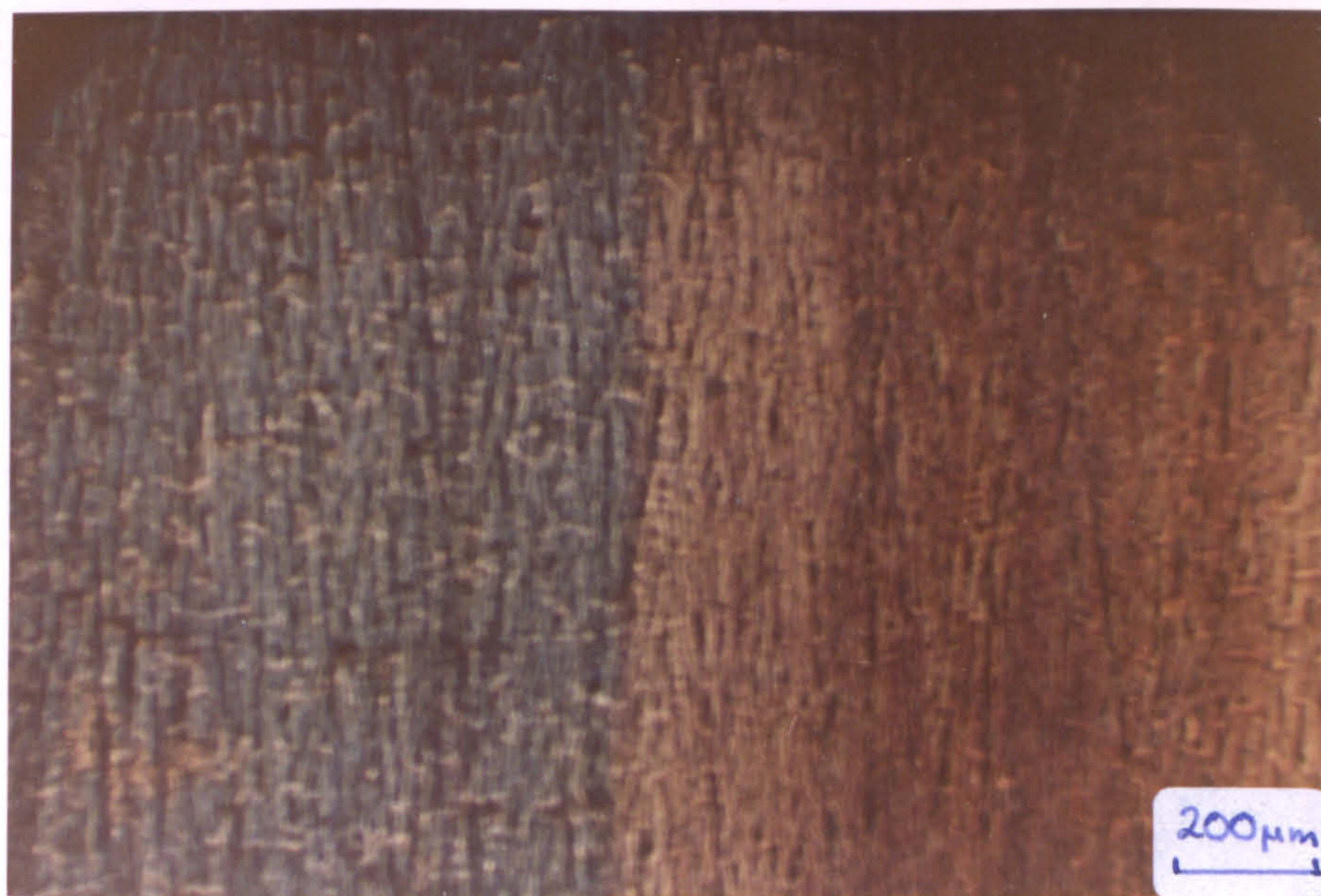
FIG. 39 Ditto- showing P.T.F.E. smeared on both ruptured and intact oxide.
