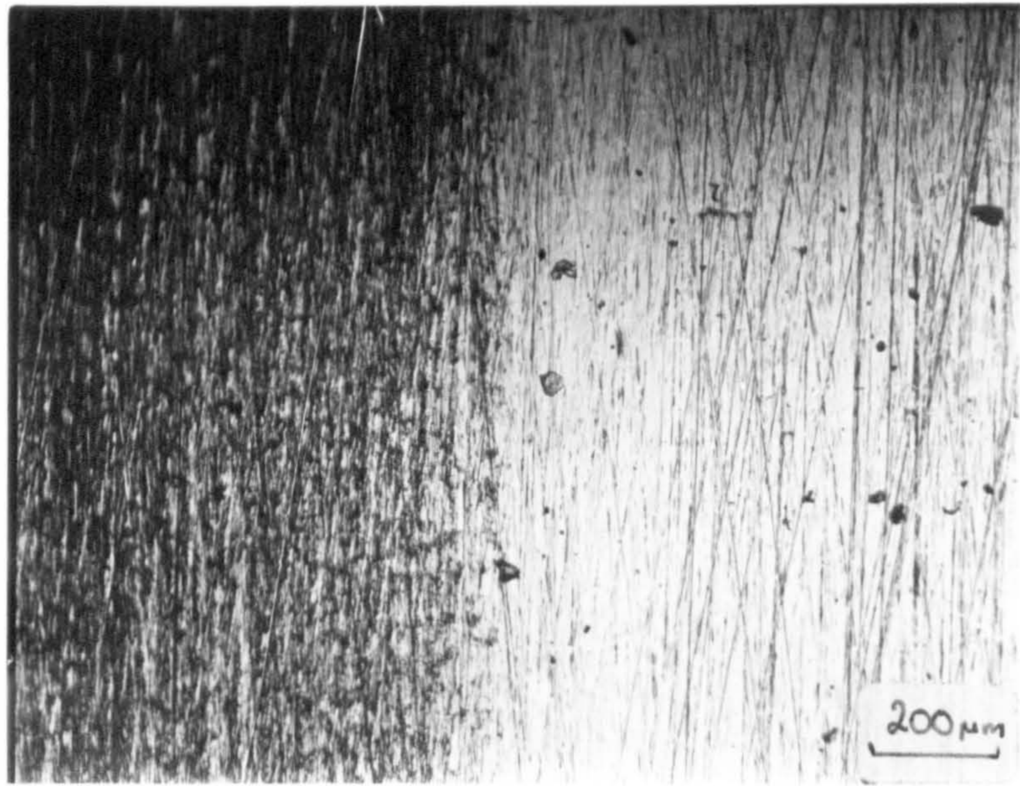
FIG. 42 Left. Smeared polymer on mild steel surface after P.C.T.F.E. had slid for 30 minutes.
