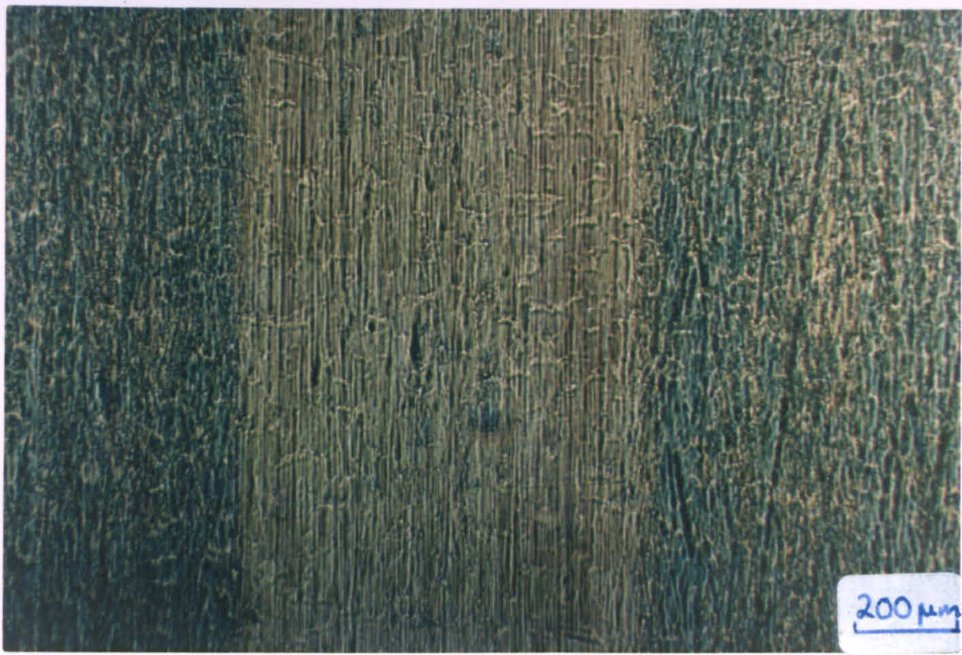
FIG. 34 Band of partially removed oxide on surface of 100nm \text{Fe}_3\text{O}_4 after P.V.C. had been sliding for 3\frac{1}{4} 10 minutes.
