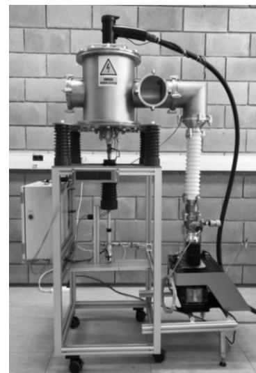
Fig. 4. Research stand based on the so-called disassemblable chamber
