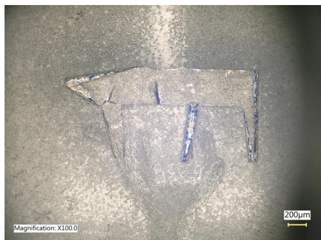
Fig. 10. Damaged nickel capacitor electrode with cells after 67 h (24 h stabilization of medium conditions and 43 h cell culture)
