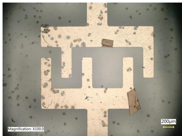
Fig. 9. Damaged nickel capacitor electrode without cells in the reference well after 67 hours (24 h stabilization of medium conditions and 43 h cell culture)
