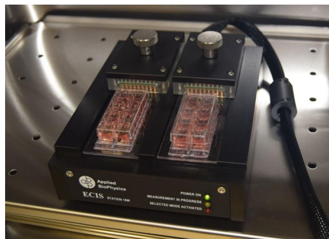
Fig. 4. The electrode array placed in the ECIS holder in the climatic chamber
