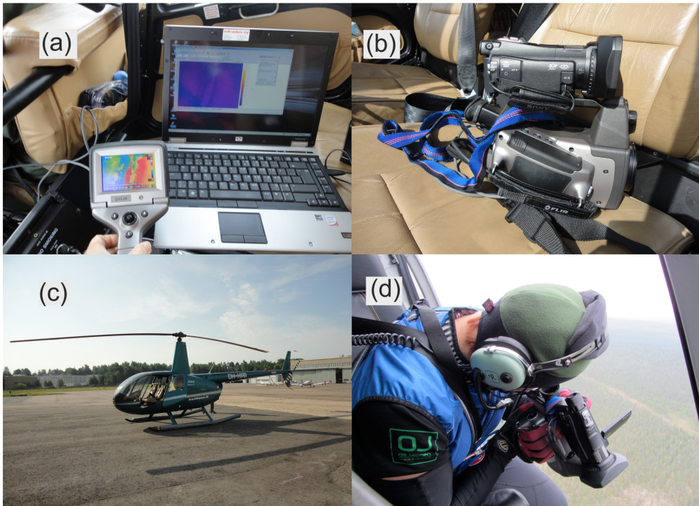
Figure 6. The low altitude aerial infrared system. (a) The on-board computer and remote control with LCD display. (b) A FLIR ThermoCAM P60 together with an HDR-CX700 digital video camera. (c) AIR surveys were acquired with A Raven R44 II helicopter. (d) The cameras held in a near vertical position on the side of the helicopter. Figures by Kirsti Korkka-Niemi. Modified from Rautio et al. 2014.
