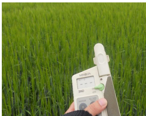
Fig. 6. SPAD-502 chlorophyll meter. Photograph by Clara Lizarazo Torres.
