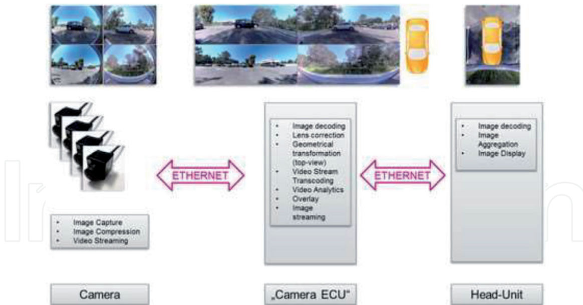
Figure 7. Video data transfer to head unit of camera through Ethernet, source: https://www.fierceelectronics.com/components/three-sensor-types-drive-autonomous-vehicles
