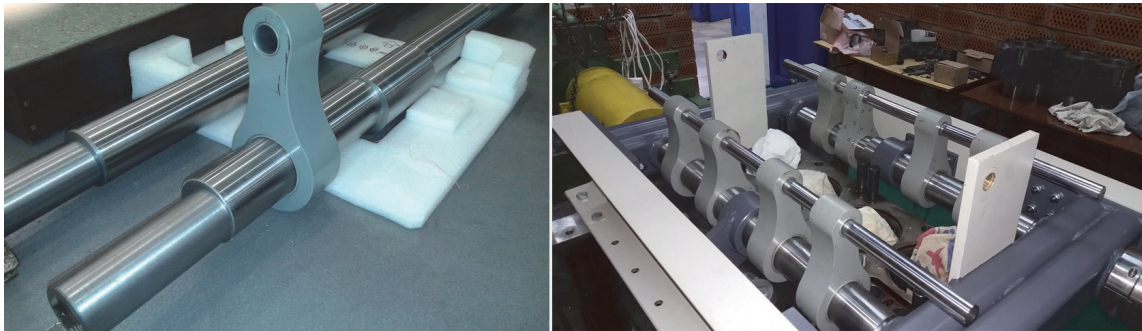
Figure 11. Connecting yokes mounted with the eccentric shafts.
