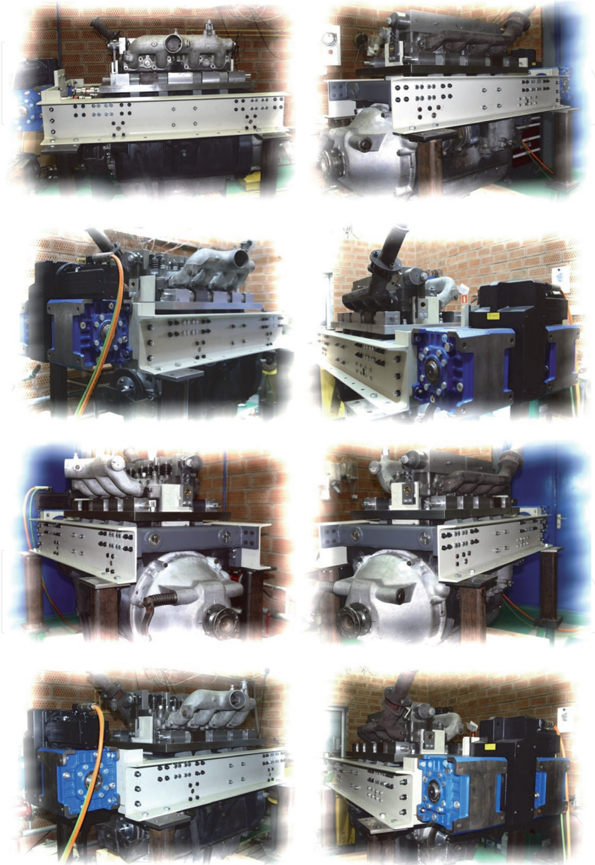
Figure 14. View of the complete VCR engine during functional tests.
