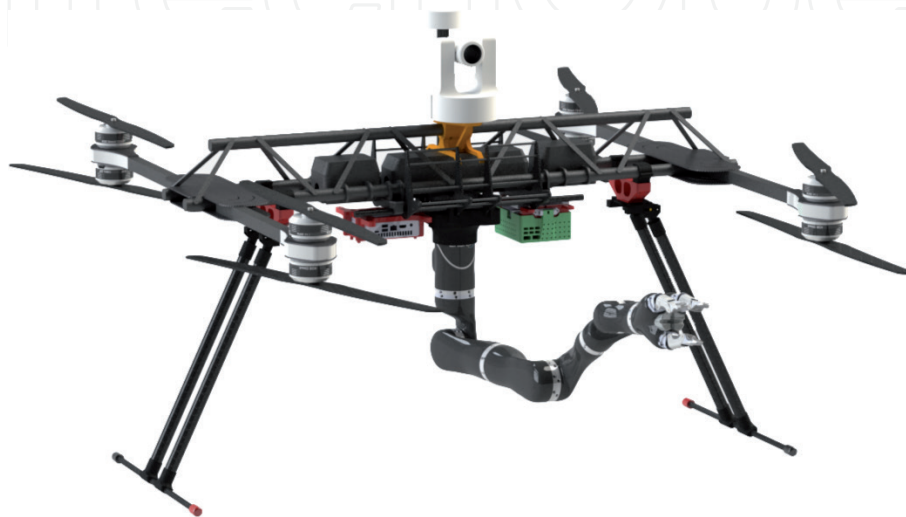
Figure 18. Aerial manipulation system with PTZ-camera.
