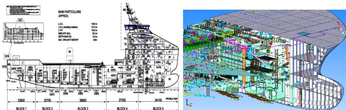
Figure 2-6: 2D vs. 3D models. Source (Vard Group AS)
