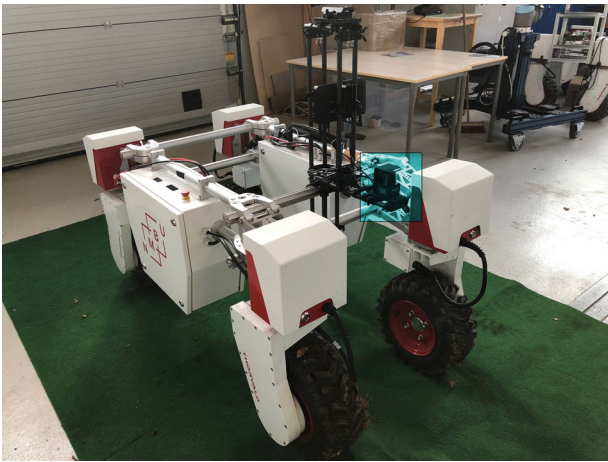
FIGURE 13 Robot setup, a 2D Hokuyo laser scanner UST-20 LX is mounted in front of the robot as shown in the highlight area [Color figure can be viewed at wileyonlinelibrary.com]
