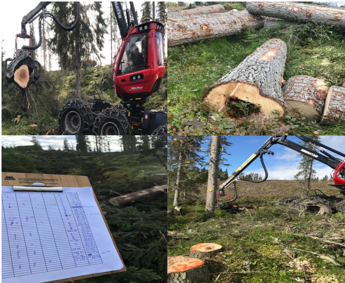
Figure 3. The work process of the second field work. First, visual inspection of trees (upper left), thereafter bucking with precision to determine the point of rot stop (upper right) and registration of the length of logs and time (lower left). Finally, marking of tree number on the stumps (lower right). The lower right photo also shows the clear-cut area with ribbon marked trees. Photos: Ole Marius Tollefsen Moen.
