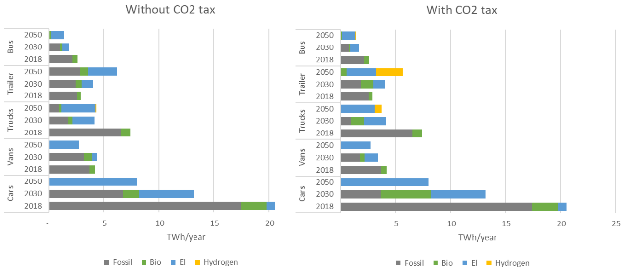
Figure 31 Energy use by energy carrier and road transport mode, TWh/year
