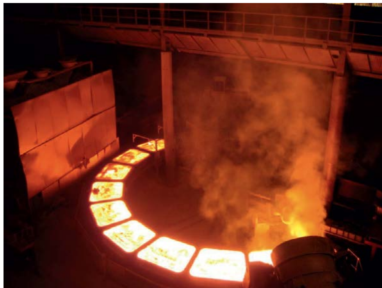
Figure 9: Casting of silicon, from [15].
