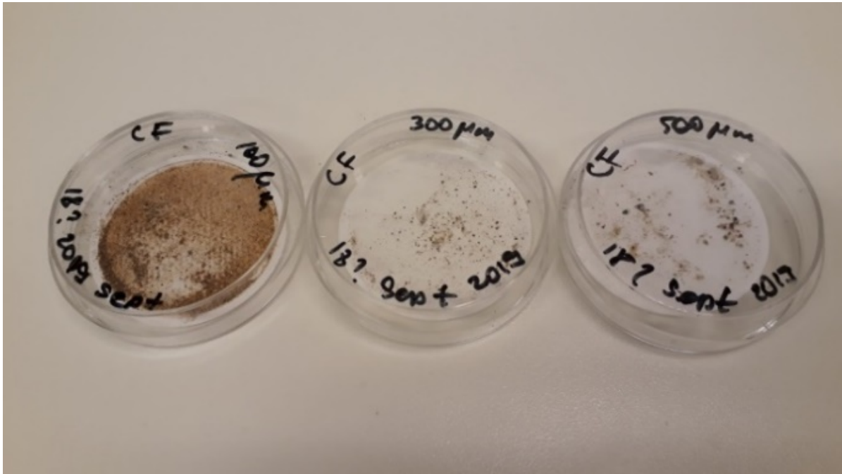
Figure 4. Example of a relatively clean sample collected on GfA filters from the 100 µm, 300 µm, 500 µm filters requiring no further pre-processing.
